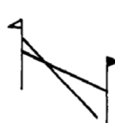
Top end of sloping pole higher than horizontal pole
